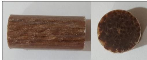
Figure 5. Kenaf composite specimen
